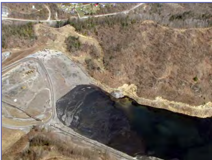
Toxic coal sludge (right), is one of the by-products of so-called "clean" coal. This particular sludge lake is held back by an earthen dam, and sits above Marsh Fork Elementary School in Raleigh County, W.Va. In 1972, a similar earthen dam failed in Logan County, W.Va. at Buffalo Creek Hollow. 125 people were killed, 1,100 injured and over 4,000 left homeless in the flood.
